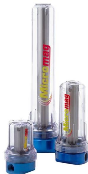
The patented, compact Micromag magnetic filter can benefit many different industries. Contaminated fluid enters the inlet port where it is dispersed by the unique tapered radial flow channels. Fluid passes down the outside of the centrally mounted rare earth magnetic core which captures contamination particles along its length, resulting in excellent filtration efficiency.
